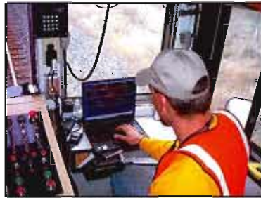
Using an eAX Wireless Workstation, Assistant Roadmaster Mike Rahl plans work, and requests and receives track authorities on a Sperry Rail Services Inspection Car
