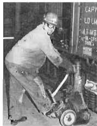
Carman Jim Spooner sets a jack in preparation for lifting a car.
