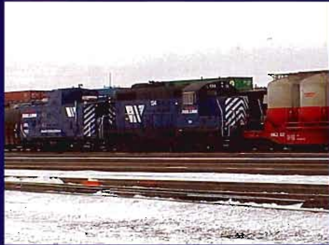
Remote Operation at Laurel Yard. Pictured here, unit 132 with Remote Control Caboose 1102, is being used to pull a cut of cars.
