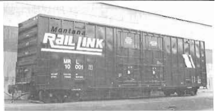
MRL 10001 at the Gunderson Plant in Portland, OR. The cars have an inside length of 50'6", inside width of 9'6" with 6,156 cubic foot capacity and are equipped with 16' double plug doors and end-of-car cushioning devices. The first car was accepted September 28.
