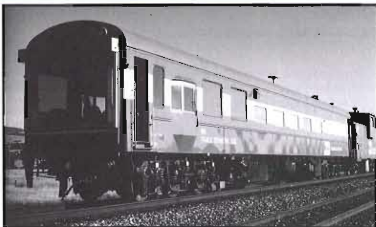
▲ BNSF B9 Track Geometry Car received extensive retrofitting with new computers and other equipment in the winter of 95-96 at the Topeka Shops. Mark Simonson photo.
