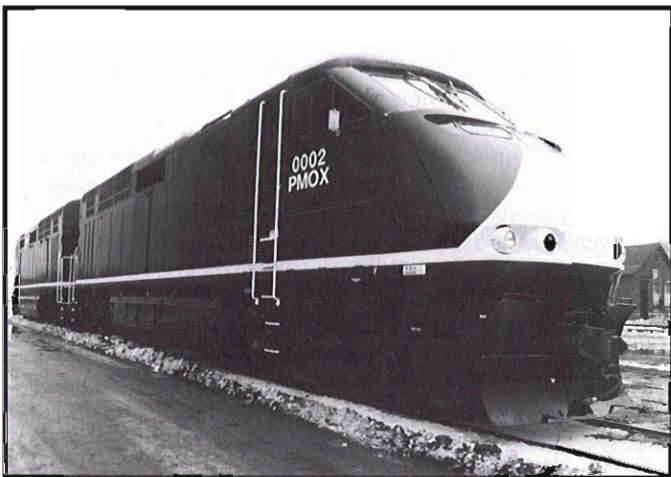
▲ Philip Morris USA plans to debut its Marlboro Unlimited luxury excursion train later this year. It will make round trips on alternating weeks between Denver and Billings, Mont., with MRL being one of the participating carriers. Two new 3,000 hp EMD F59PHI locomotives, pictured here just off the assembly line in London, Ont., will pull the train. Rader Rail Car of Denver, is building the cars for the train. Photo courtesy Philip Morris USA.
