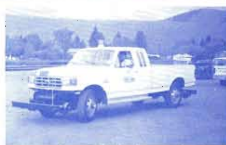
A 1988 Ford F-260 Supercab pickup truck with 4-wheel drive and hyrail assigned to Helena roadmaster Pete Christensen (in cab) typifies the new vehicles acquired this year.
