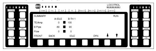
If the consists were operating in power or dynamic braking (synchronous) when the rear remote consist was moved to the back group, the rear remote will remain at its present power setting until it is changed using the soft keys on the Summary screen.
