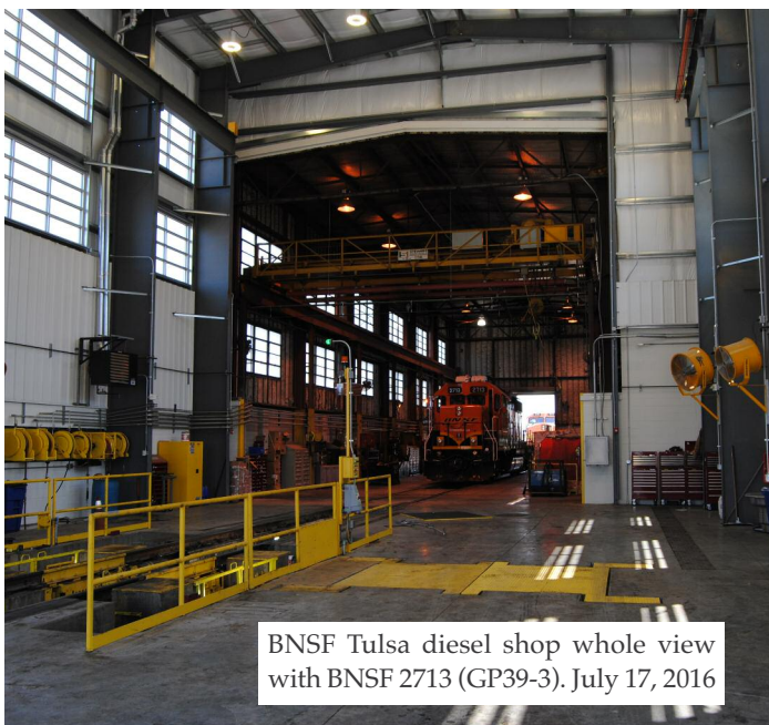
The drop table is used to lower and raise traction motors so they don't have to lift locomotives. July 17, 2016.
