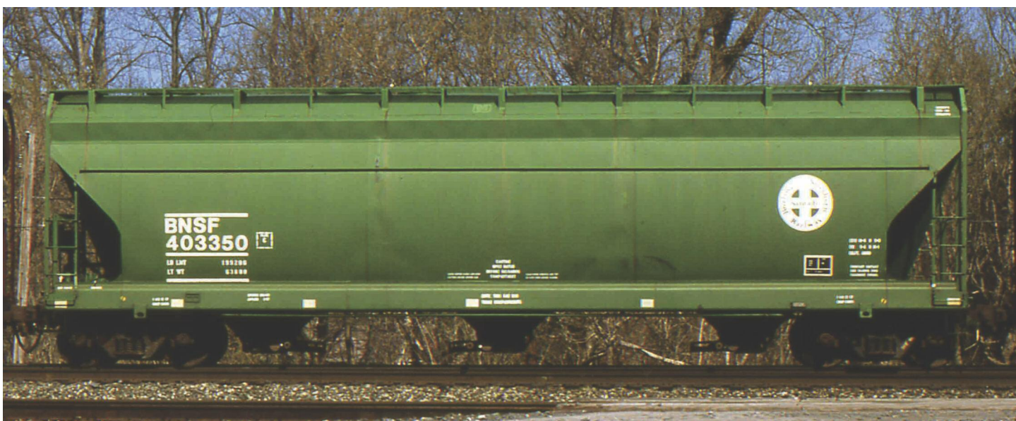
BNSF 403350, ACF, 4650 cf, at Berea Ohio, on NS, on April 19, 2007. Photo by Mark Demaline.
