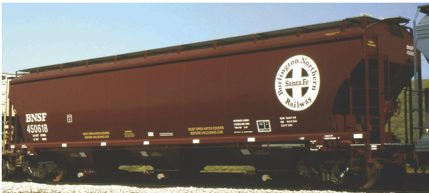
BNSF 450618, Johnstown America, 5161 cf, blt 2000, at Wellington Ohio, on CSXT, July 2001. Photo by Mark Demaline.
