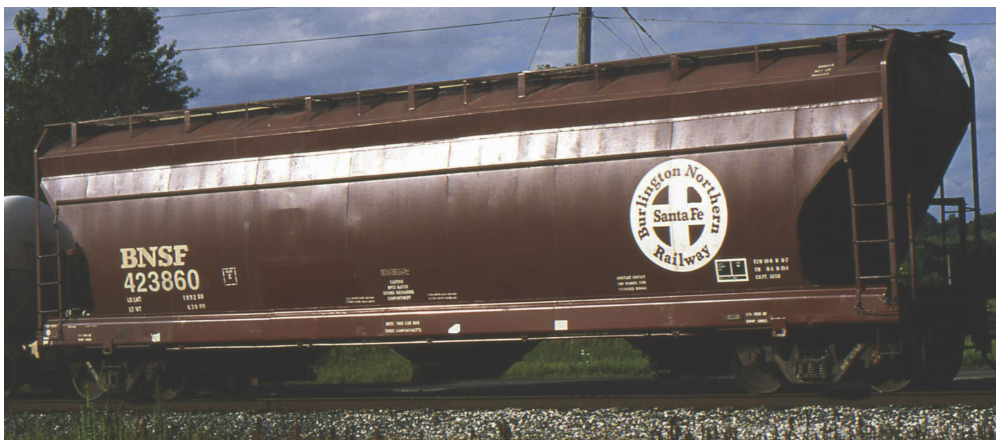
BNSF 423860, ACF, 4650 cf, blt 1966. Ex-GN. At Sterling Ohio, on CSXT, August 2, 1004. Photo by Mark Demaline.
