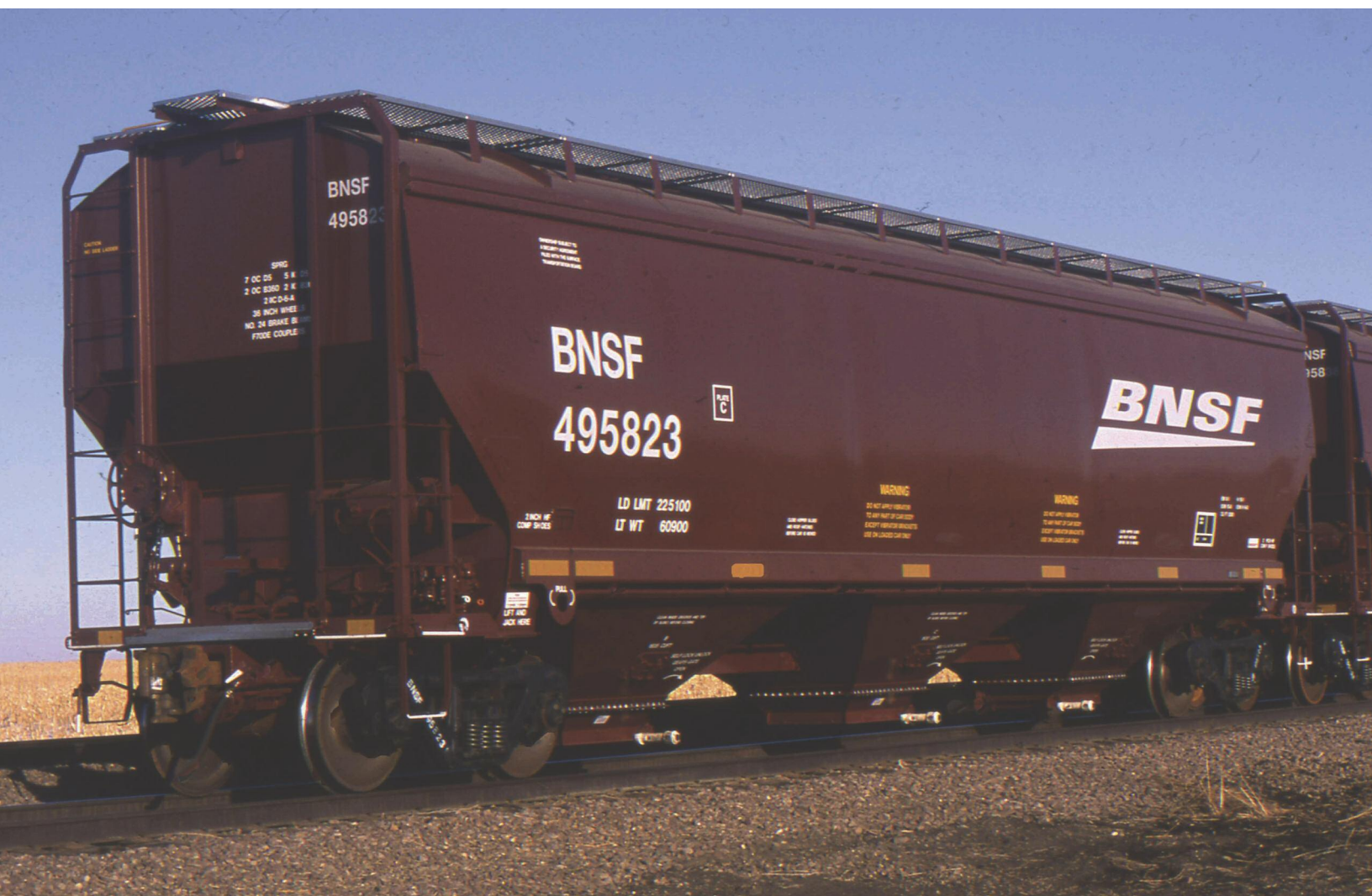
Almost new BNSF 495823, 5200 cf, blt by Gunderson in October of 2014. Both photos taken on January 18, 2015 in Beebe, South Dakota by Jeff Hendricks.
