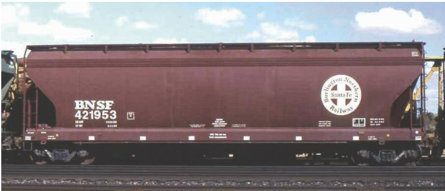
BNSF 421953, ACF, 4650 cf, at Shelby Montana on BNSF, October 8, 2001. Photo by Mark Demaline.
