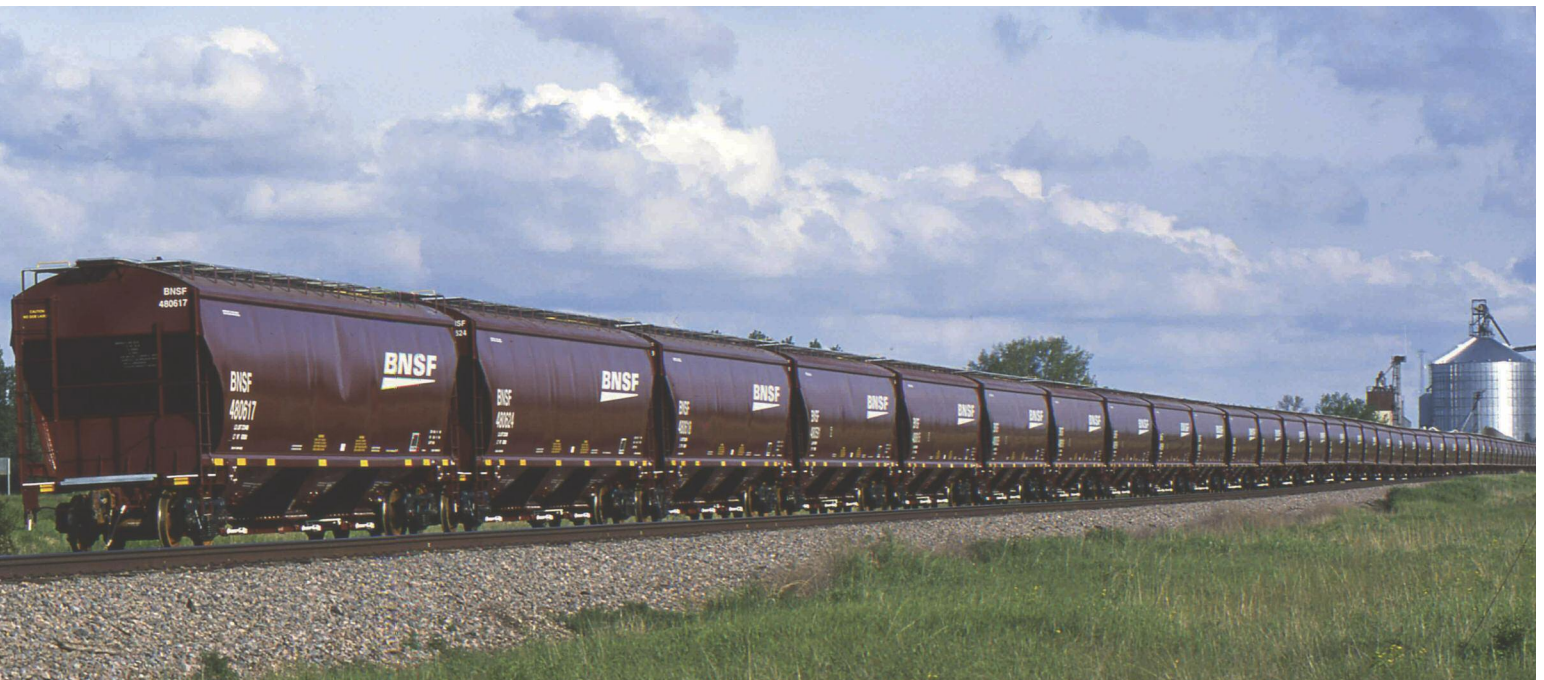
A train of brand new "Swoosh logo" cars, including BNSF 480617, is near Morris Minnesota, on the BNSF. It is June 7, 2005, and these 5161 cf cars have just arrived from builder Trinity Industries for their first load cycle. Photo by Mark Demaline.
