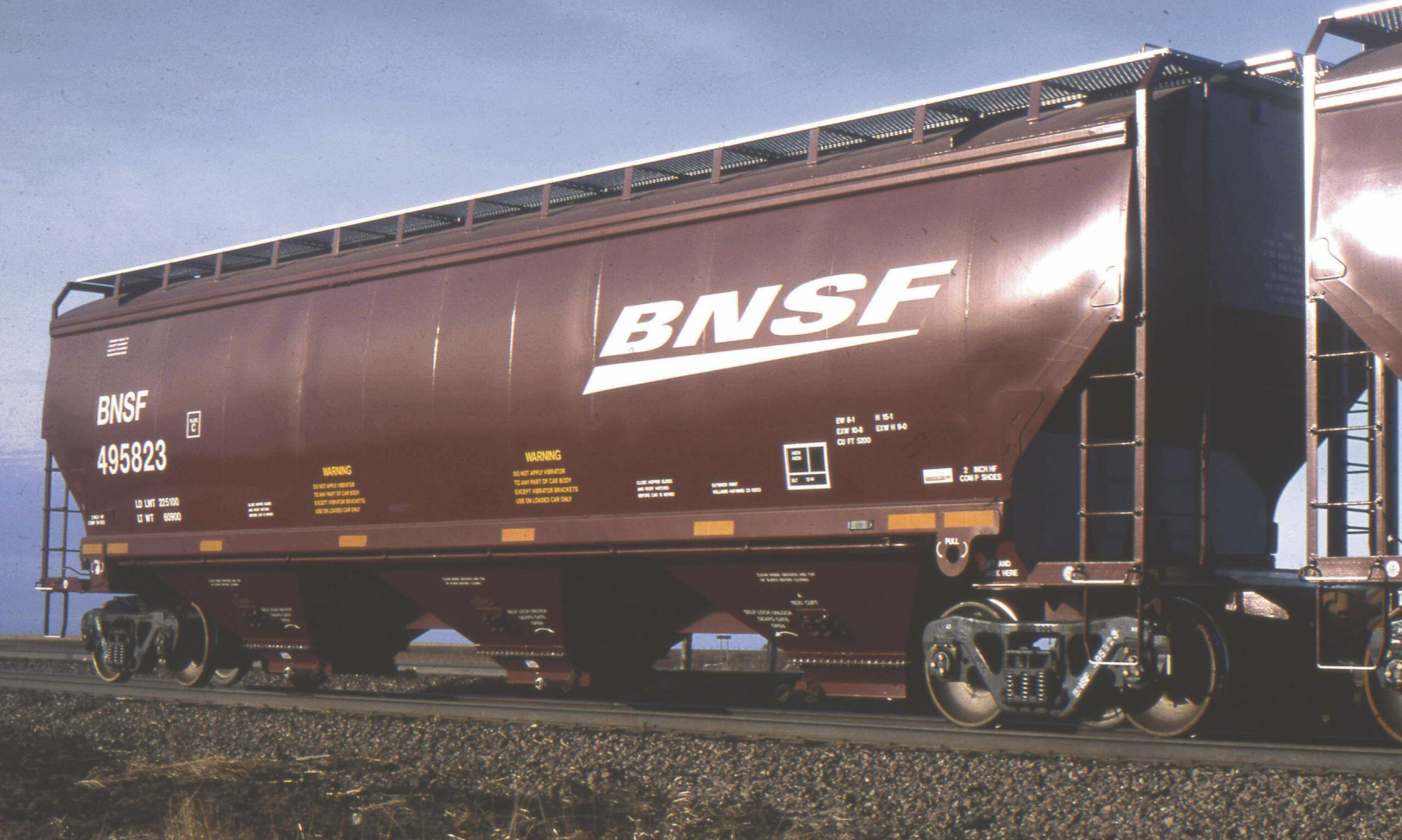
Almost new BNSF 495823, 5200 cf, blt by Gunderson in October of 2014. Both photos taken on January 18, 2015 in Beebe, South Dakota by Jeff Hendricks.
