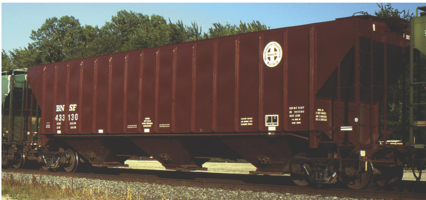
BNSF 433130, P-S Butler, 4740 cf, blt 1967-68, at Grafton Ohio, on CSXT, July 8, 2001. Photo by Mark Demaline.
