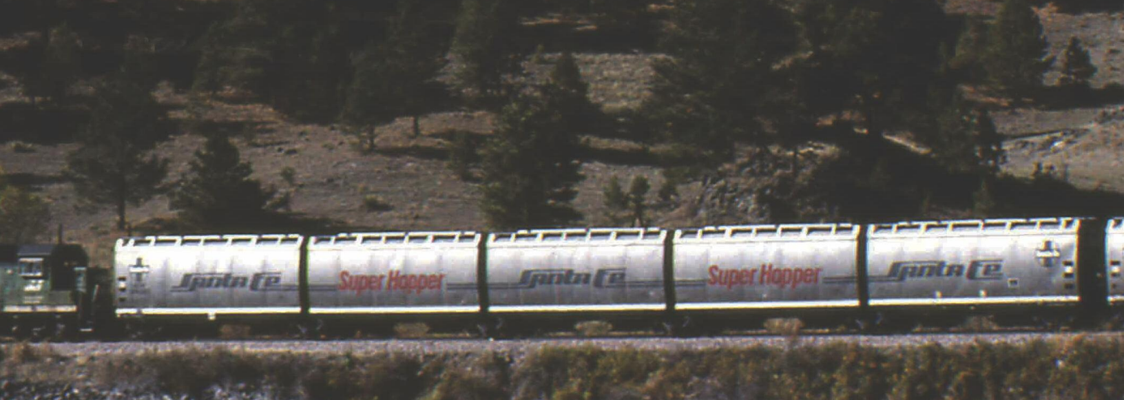
ATSF 39001-39002, 2 of 3 "Super Hopper" articulated cars, built by Thrall. Each car had 16,200 cf capacity and was 166'7" long. They were loaded at Conrad Montana on BNSF, and here westbound on BNSF at Craig Montana, October 13, 1999. Below is a close-up of one of the units in Conrad two days prior. The cars remained in service at least until 2007. Both photos by Mark Demaline.
