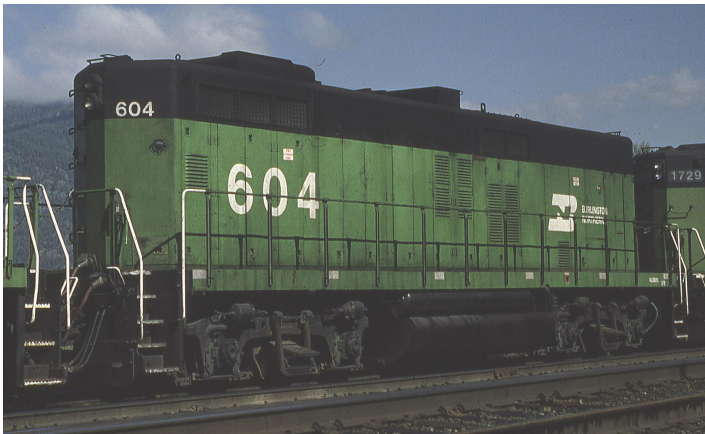
GP9B 604 was rebuilt as a cabless (booster) from GP9 1818 in 1982. Brian Ambrose photographed it (above) in Sandpoint, Idaho on May 8, 1986. Shortly thereafter it was modified for use as a shop switcher at the Havelock car shops by adding a makeshift cab and equipping it for remote-control operation. It was designated as "RC Control Derrick, Locomotive" in BN's roster. The photo below shows it at work in Lincoln, Nebraska on March 13, 1998. Photo by Jim Shepard from the Keith Ardinger collection.
