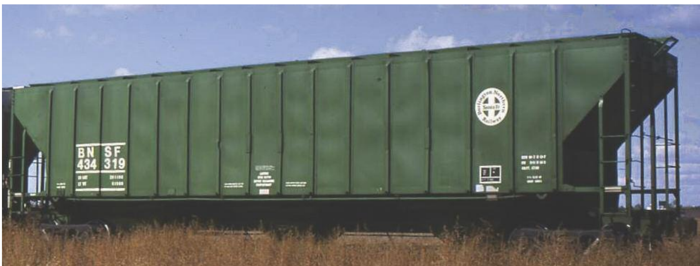
BNSF 434319, P-S Butler, 4740 cf, blt 1967, at Shelby Montana, on BNSF, October 8, 2001. Photo by Mark Demaline.
