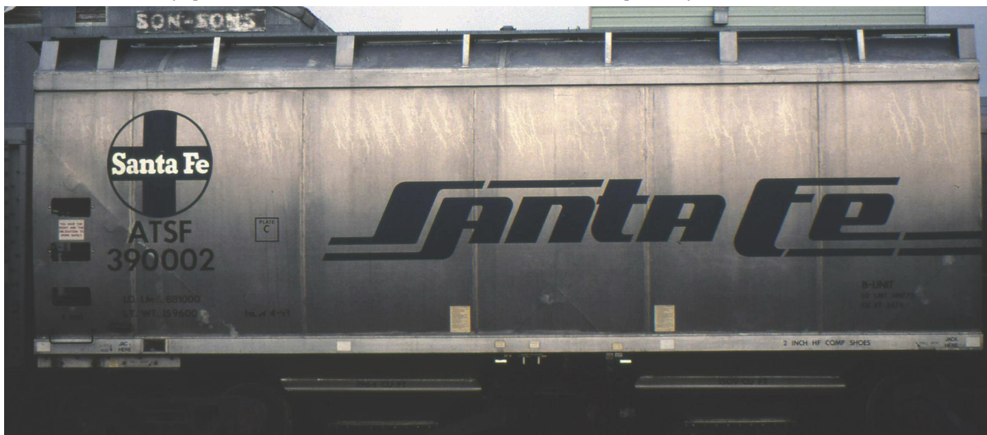
ATSF 39001-39002, 2 of 3 "Super Hopper" articulated cars, built by Thrall. Each car had 16,200 cf capacity and was 166'7" long. They were loaded at Conrad Montana on BNSF, and here westbound on BNSF at Craig Montana, October 13, 1999. Below is a close-up of one of the units in Conrad two days prior. The cars remained in service at least until 2007. Both photos by Mark Demaline.
