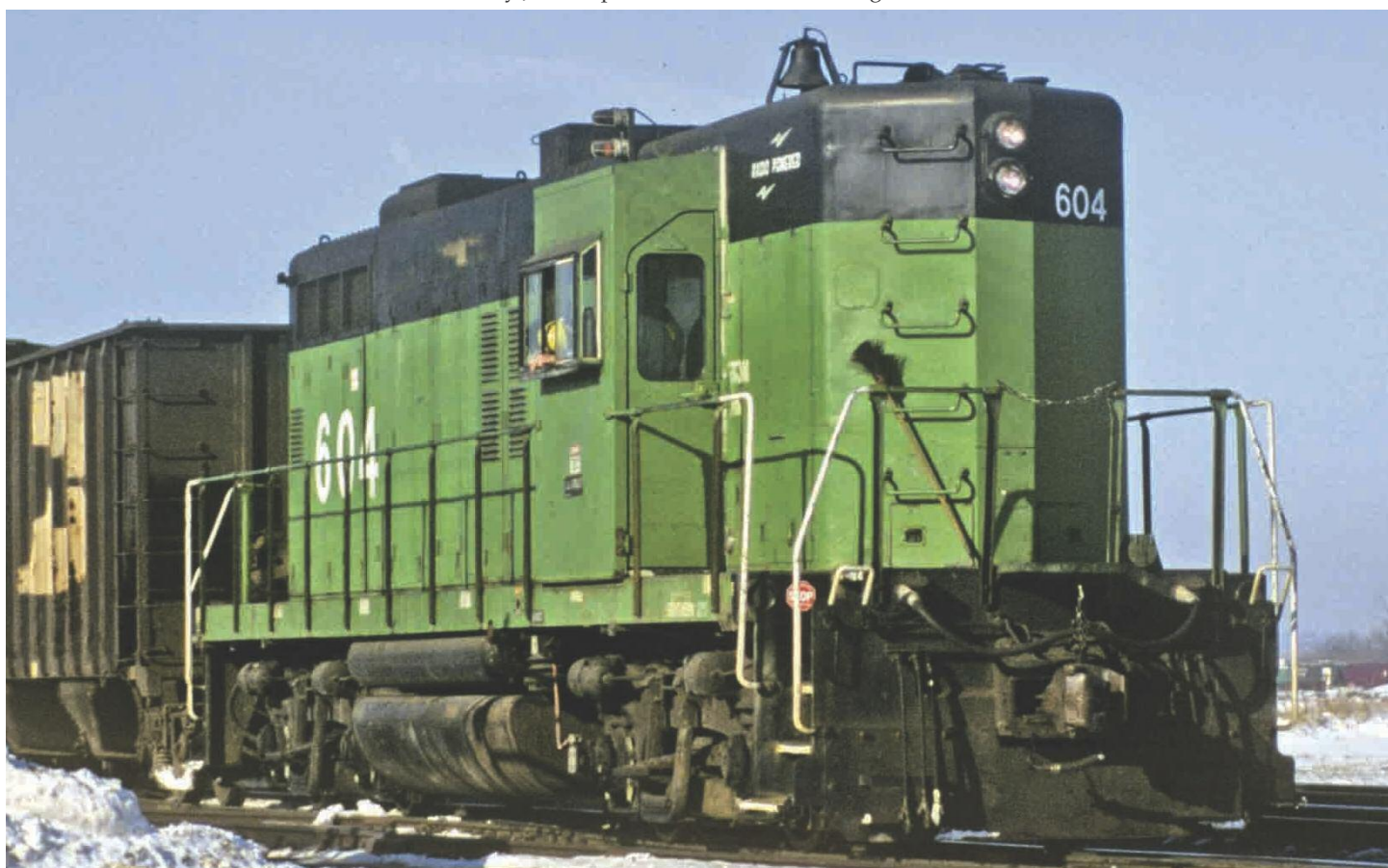
GP9B 604 was rebuilt as a cabless (booster) from GP9 1818 in 1982. Brian Ambrose photographed it (above) in Sandpoint, Idaho on May 8, 1986. Shortly thereafter it was modified for use as a shop switcher at the Havelock car shops by adding a makeshift cab and equipping it for remote-control operation. It was designated as "RC Control Derrick, Locomotive" in BN's roster. The photo below shows it at work in Lincoln, Nebraska on March 13, 1998. Photo by Jim Shepard from the Keith Ardinger collection.
