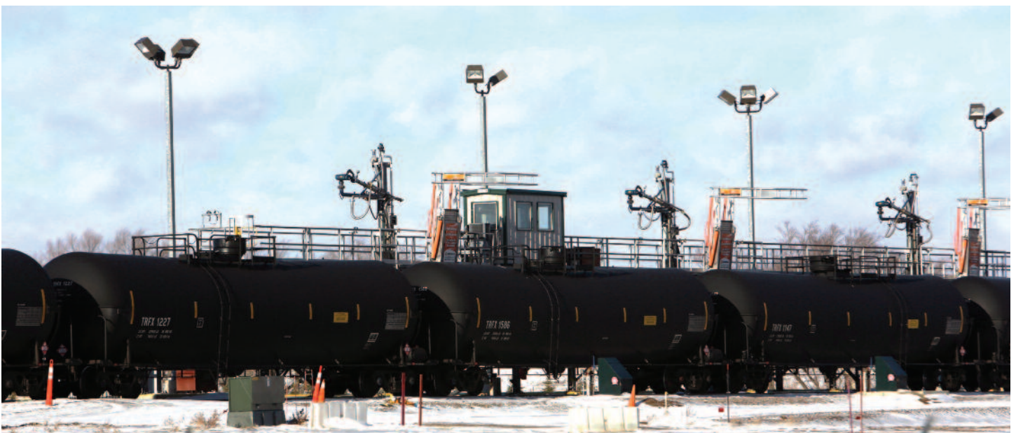
(below) A close-up view of the loading racks shows many details of the oil transfer equipment currently in the retracted position.
