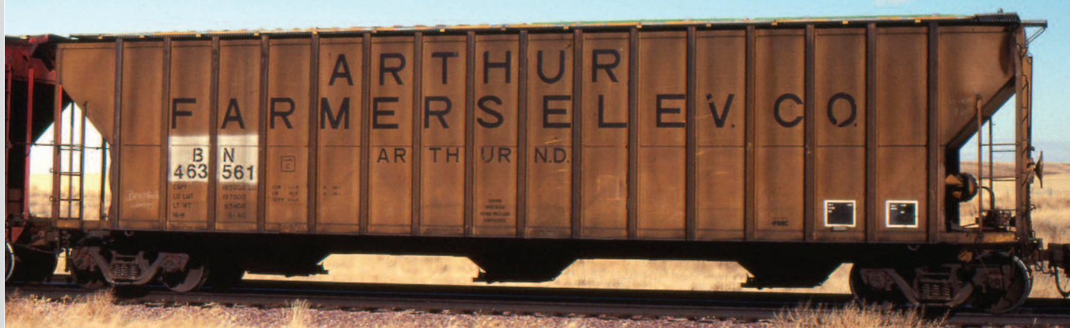
BN 463581, an ex-Arthur Farmers Elevator car, FMC, 4750 cf, blt 1980, Eastham Jct MT on the BNSF, October 12, 1999. Mark Demaline photo.
