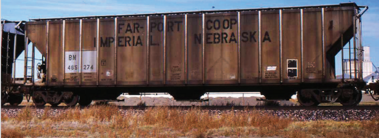
An ex-Far-Port Coop car, BN 465274, built by Evans, 4780 cf, at Shelby MT on the BNSF, October 3,2001. Mark Demaline photo.
