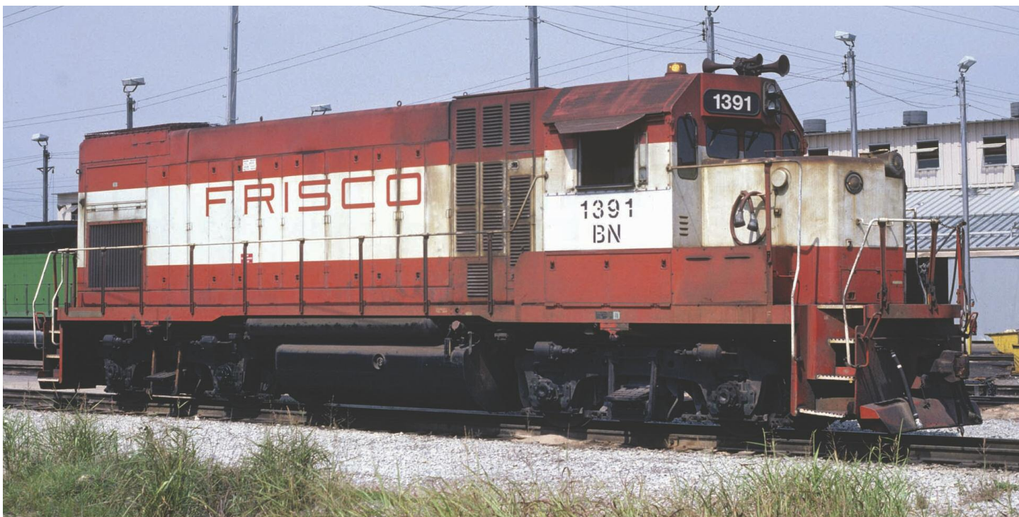
(above) Ex-Frisco GP15-1 1391, shown here in Omaha, Nebraska on September 12, 1981, is an example of how the units were renumbered by painting over the exiting Frisco number below the cab window and stenciling on BN and the new number. The bright white paint stands out next to the grimy exterior of the rest of the unit. Photo by David M. Johnson, from the Keith Ardinger collection.
