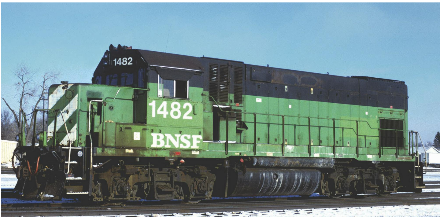
(above) GP15-1 1482, one of only two left on the BNSF roster as of 2014. The unit is basking in a warm winter's sun in Grand Forks, North Dakota on January 17, 2002. Note that the nose-mounted gyralite has been removed and the mounting notch welded over. Photo by Pat Monahan, from the Keith Ardinger collection.
