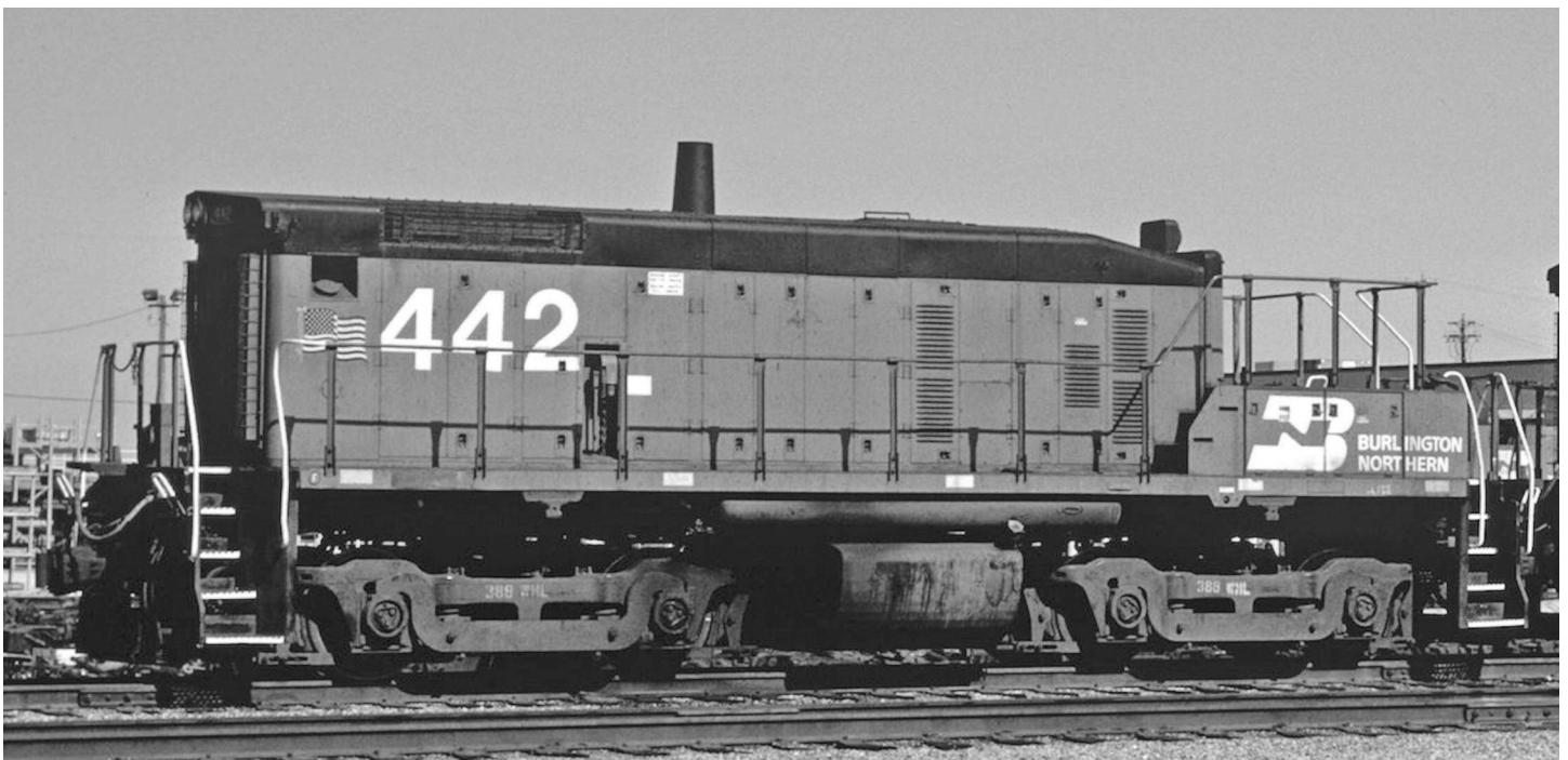
SW10 442 was rebuilt at West Burlington into an SW10B in January 1987 after suffering cab damage. Galesburg, Illinois on July 18, 1992. Photo by Jim Shepard, from the Keith Ardinger collection.
