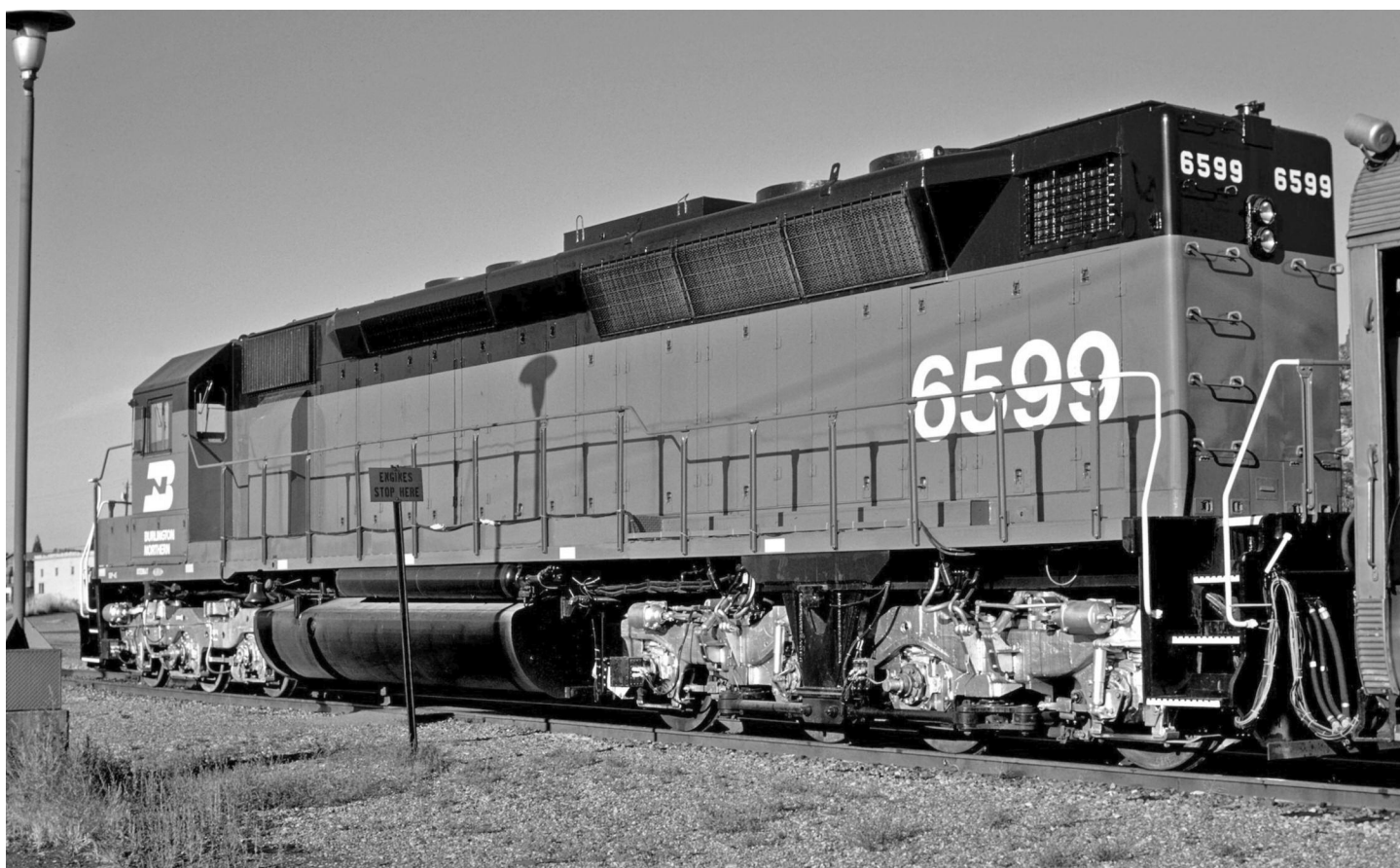
(below) Number 6599 was the most unusual SDP45 on BN's roster. EMD replaced the rear 3-axle truck with an experimental 4-axle radial guide self-steering truck in 1984. The original truck was put back in early 1987, after which this unit and all remaining SDP45's on the roster were retired and sold. Auburn, Washington, September 16, 1984. Photo by Scott O'Dell, from the Keith Ardinger collection.
