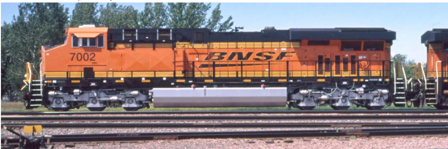
(below) BNSF 7002 (ES44C4) at Aberdeen, SD on June 11, 2012. Built 4/12/2012, serial 60936. Unit has 43" wheels and meets Tier III. -both photos by Jeff Hendricks
