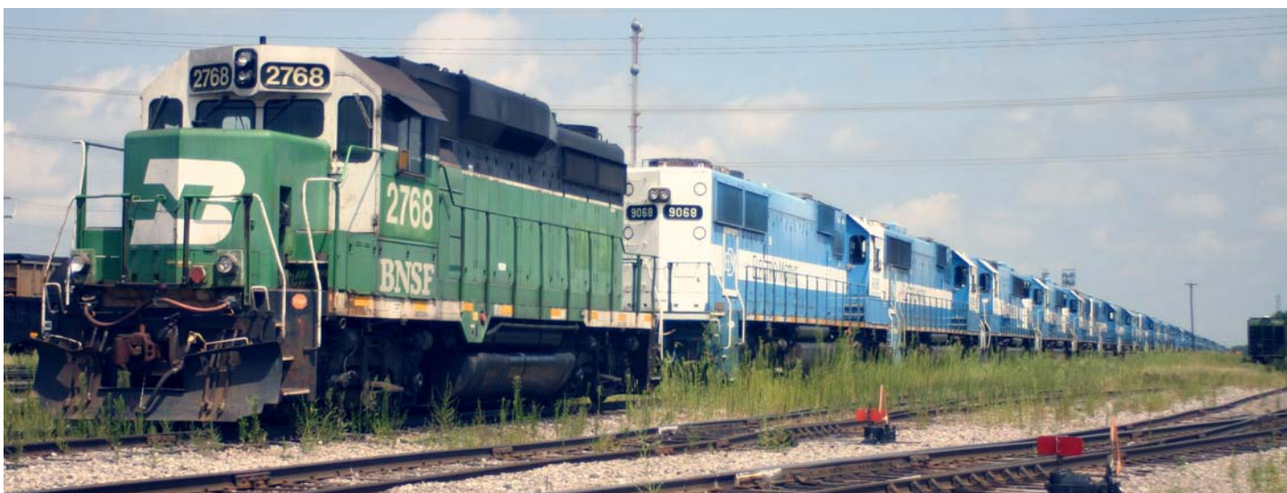
(center) On August 9, 2010, the 2768 sits at Creston, IA, with a string of Oakway units. The 2768 is a GP39-2R, it has a GP30 carbody and a GP39 cab. Built in October 1963 as Southern GP302591, the "R" designates a 16-cylinder engine instead of the standard 12-cylinder engine. -Patrick Lana photo
