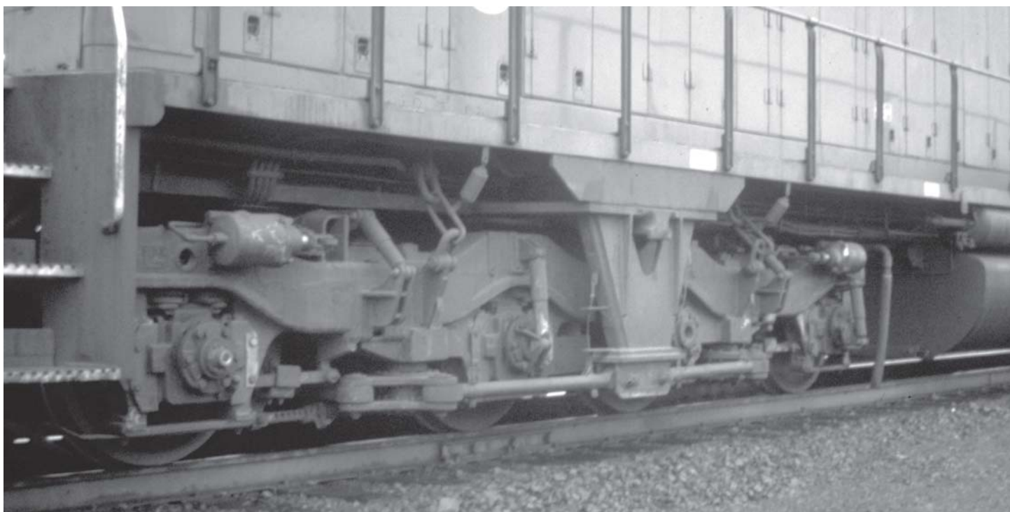
Close-up of 6599's 4-axle truck. Vancouver, WA. -Roland Haynes photo
