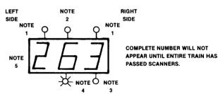
Note 1—Hot bearing indicator light. When illuminated hot bearing detected. The hot bearing is located on right side of train when right light is illuminated, and on left side when left light is illuminated.
