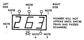
Note: 1—Hot bearing indicator light. When illuminated hot bearing detected. The hot bearing is located on right side of train when right light is illuminated, and on left side when left light is illuminated.
