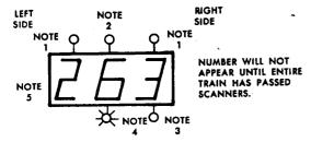
Note: 1—Hot bearing indicator light. When illuminated hot bearing detected. The hot bearing is located on right side of train when right light is illuminated, and on left side when left light is illuminated.
