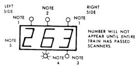
Note: 1—Hot bearing indicator light. When illuminated hot bearing detected. The hot bearing is located on right side of train when
