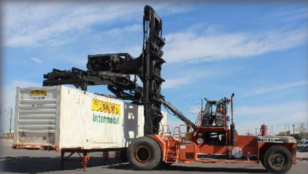
1. Crane "grabs" container and trailer at lift points.
