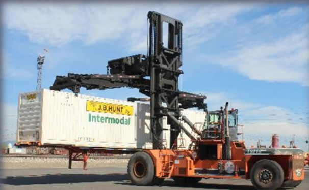
4. With trailer raised, crane begins turn to reposition trailer.
