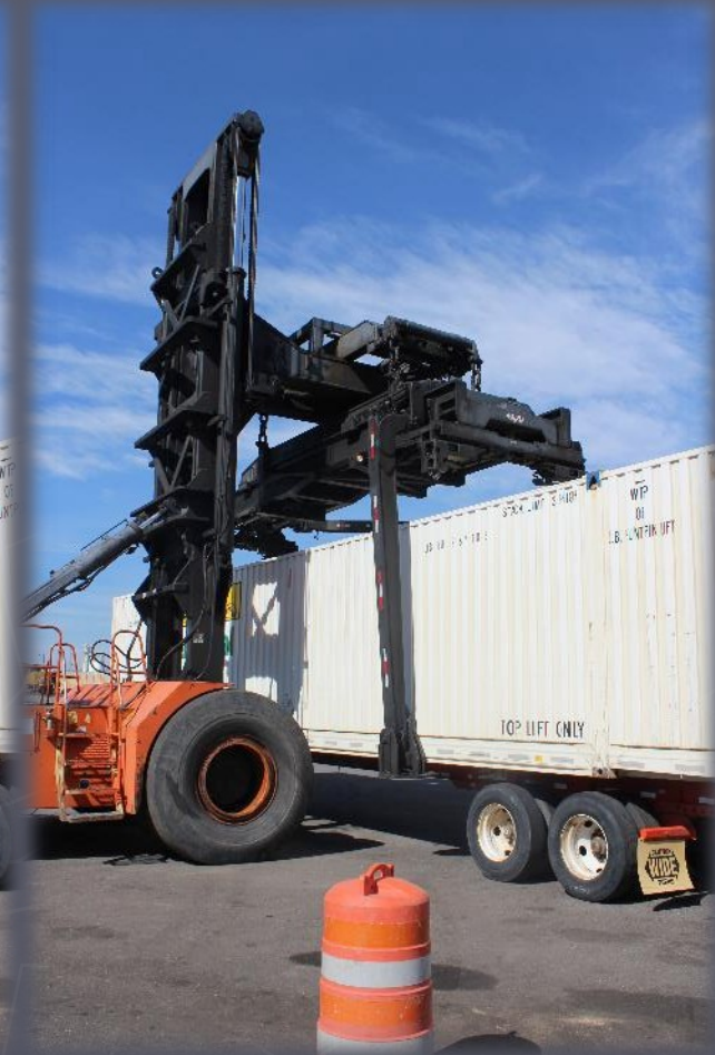
3. Crane arms now dropped on both sides of trailer and can begin to lift.
