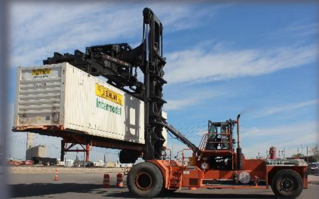
3. Crane lifts container and trailer to full height.
