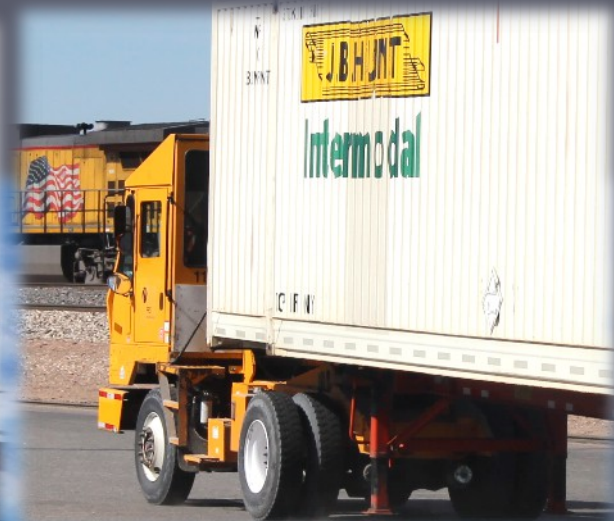
3. Yard Dog pulling trailer to assigned spot with hydraulic fifth wheel keeping the trailer landing gear off ground.
