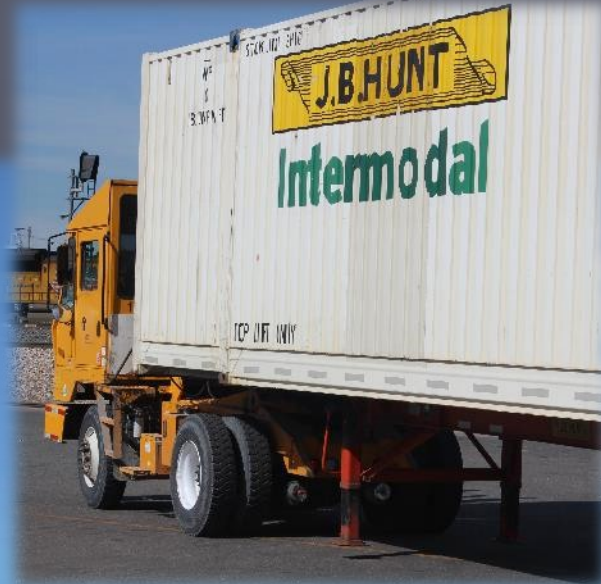
2. Yard Dog coupled to trailer. Driver attaches air hoses and raises landing gear with hydraulic fifth wheel.
