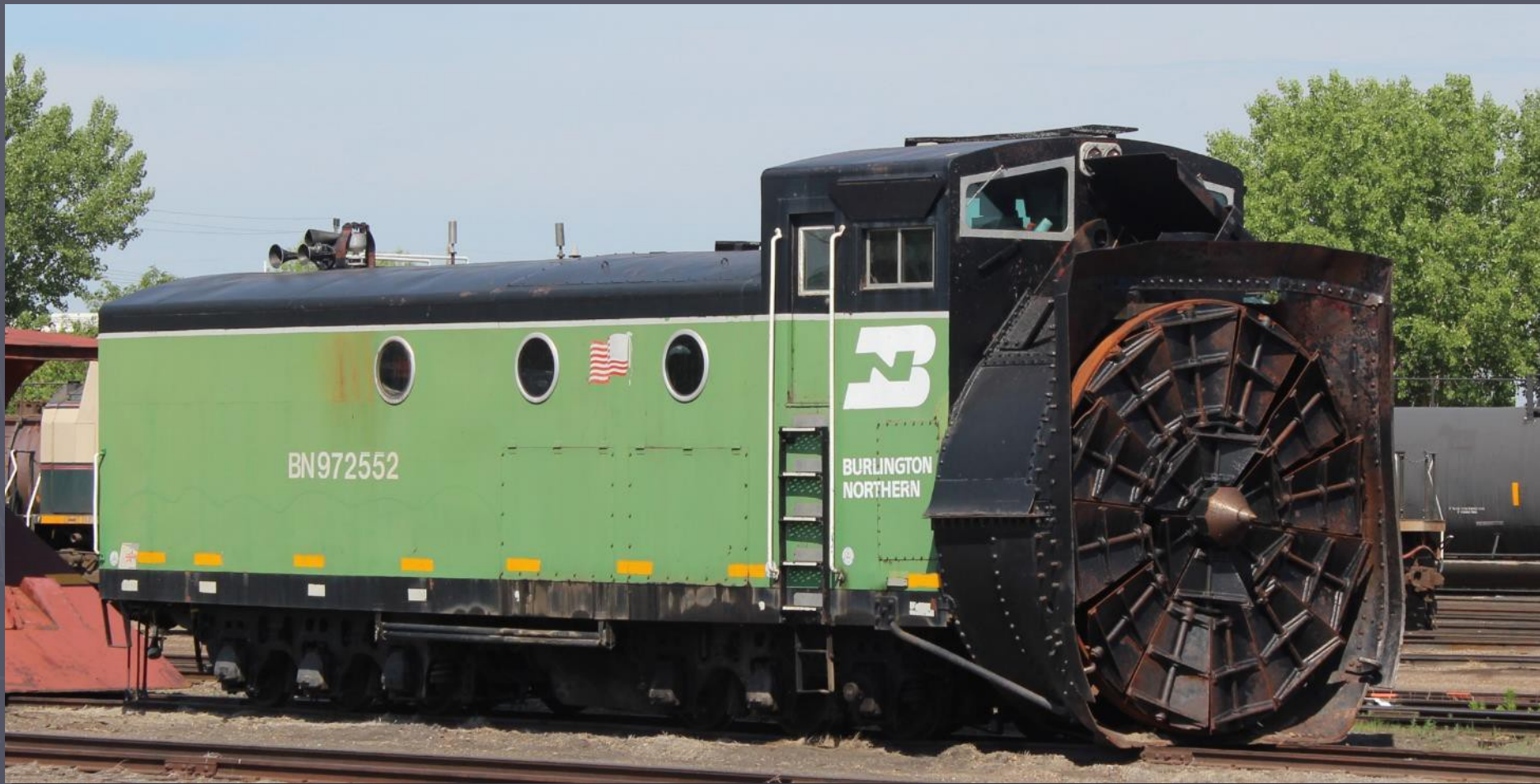
Rotary Snowplow BN 972552 former GN X-1507, Built 1907 by Alco, Rebuilt 1963 on tender frame. Source: http://www.trainweb.org/rrsnowfighting/bnsf.htm Glendive, MT Yard Tour
