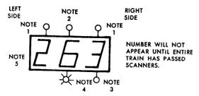
Note: 1—Hot bearing indicator light. When illuminated hot bearing detected. The hot bearing is located on right side of train when right light is illuminated and on left side when left light is illuminated. Stop and inspect train.
