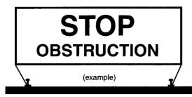
This banner is considered a stop signal and a simulation of ontrack equipment. Whenever required by an operating rule, stop all train, engine, and on-track equipment movements short of the "STOP" or "STOP OBSTRUCTION" banner.
